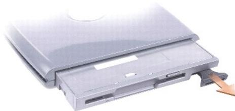
5. Insert the new device into the bay, push the device until you feel a click, and push the device latch release in so that it is flush with the bay.
