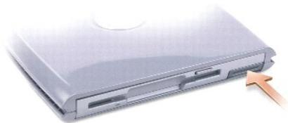
4. Pull the device by the latch release to remove the device from the D/Bay.
