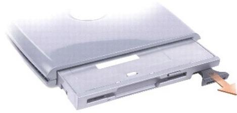
5. Insert the new device into the bay, push the device until you feel a click, and push the device latch release in so that it is flush with the computer.
