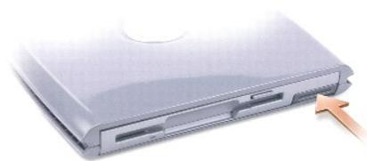
2. Pull the device by the latch release to remove the device from the D/Bay.
